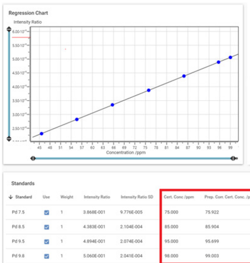
Figure 6: Example of a calibration function with the corrected standard concentrations calculated using actual preparation amounts
